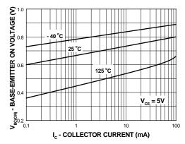
Figure 4. Base-Emitter On Voltage vs.Collector Current
